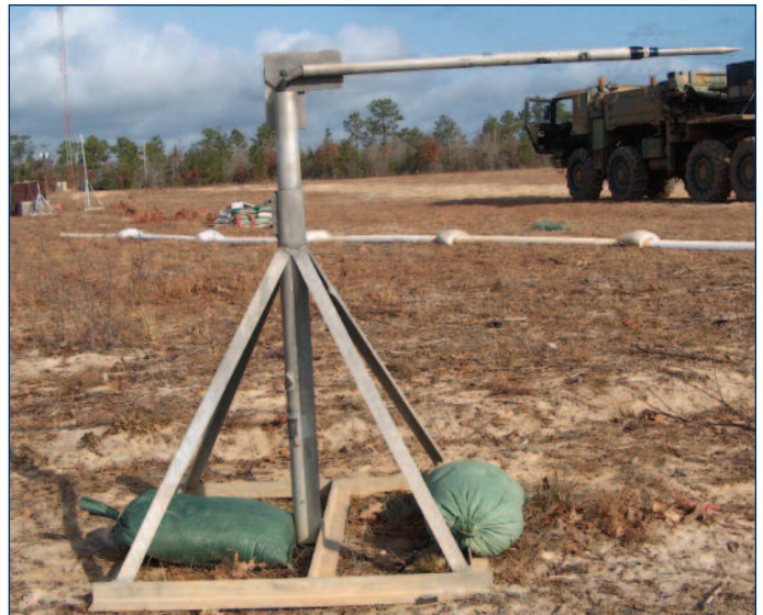
FIGURE 3: Pencil Probe Field Application
